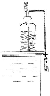
in our laboratory. In the course of some experiments with sand filters, samples of the different effluents as well as of the applied sewage were taken daily, treated with a small quantity of a concentrated sterilizing agent, and an analysis made each week of the combined daily samples.
